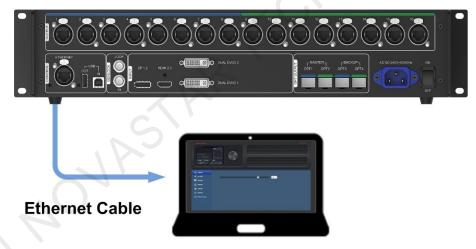
Step 2 Connect the MCTRL4K to a PC (or a mobile device) via Ethernet cable or router.
