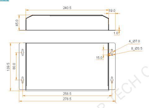
Tolerance: ±0.1 Unit: mm
