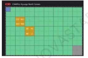
You can click on the abnormal module in the topology and enable **Cabinet Finder** or **Module Finder** function in the **Cabinet Settings** area to quickly find the cabinet or module where the LED errors or abnormal LEDs are located.
