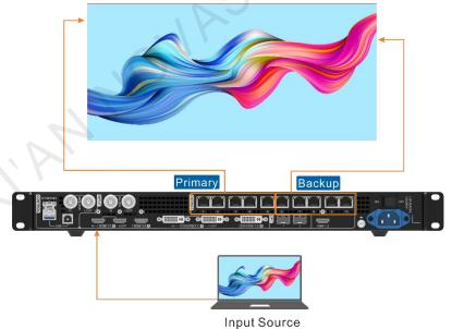
The setting procedure for the Ethernet port backup:
