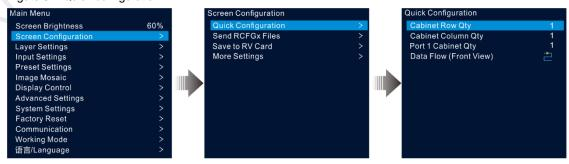
Step 3 Rotate the knob to select Port 1 Cabinet Qty to set the quantity of the cabinets loaded by Ethernet port 1.
