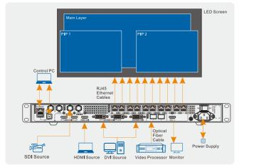
· Work as a fiber converter for long-distance transmission
