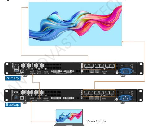
The setting procedure for the device backup:
