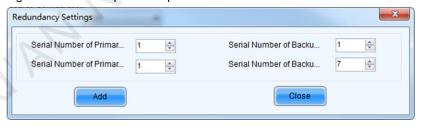
Step 7 Click **Add** to complete the backup settings of an Ethernet port, and the system will automatically list the primary ports and backup ports.
