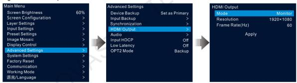
Step 2 Rotate the knob to select **Mode** to set the HDMI output connector mode.
