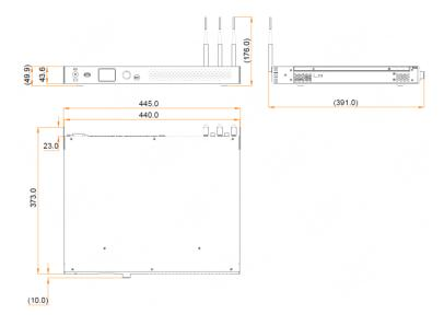
Tolerance: ±0.3 Unit: mm
